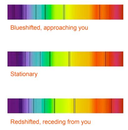
The amount of shift you get depends on the velocity: faster objects have the spectral lines shifted further from the rest wavelength.
